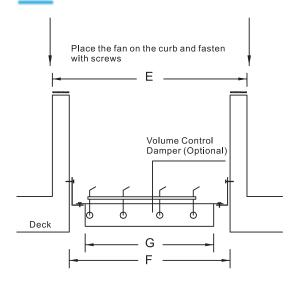
The height of the curb (H) is generally identified by the design engineer. A 300 mm-500 mm range is recommended and can be chosen within the range based on the amount of local rainfall.
